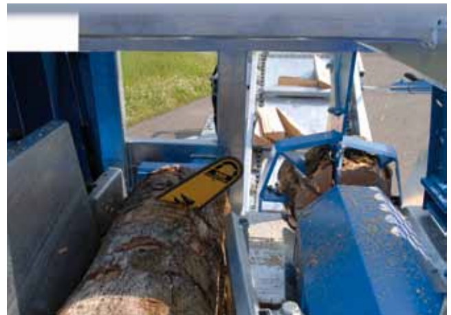
Links: Harvester-Schwert, rechts: Spaltkanal
